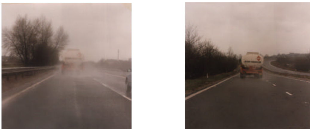
Figure 10.1: Examples illustrating splash and spray from a truck driving on dense and porous asphalt respectively. [105]
