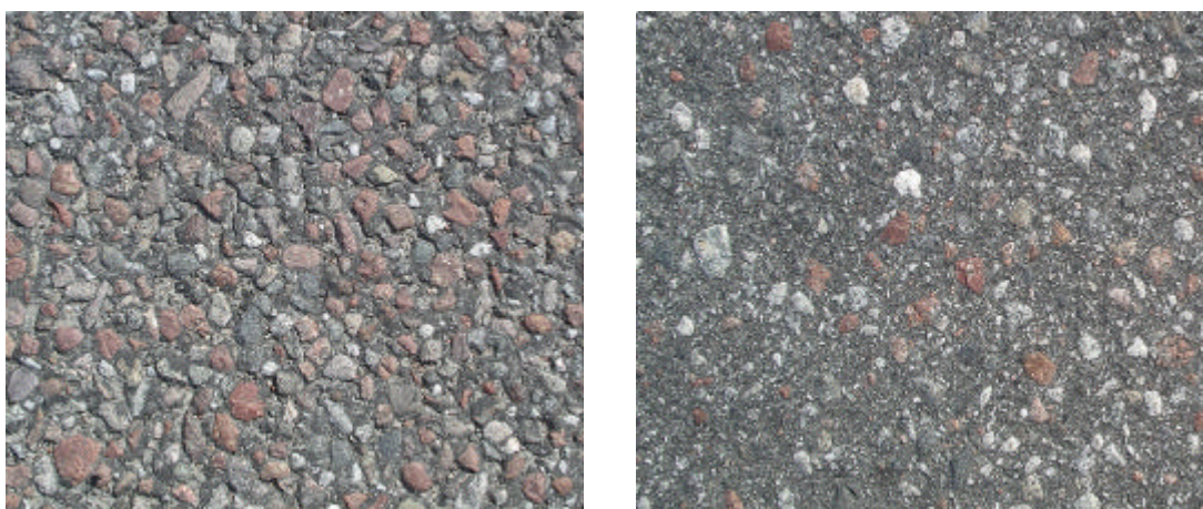
Figure 4.4: Comparison of surface texture of SMA and AC
