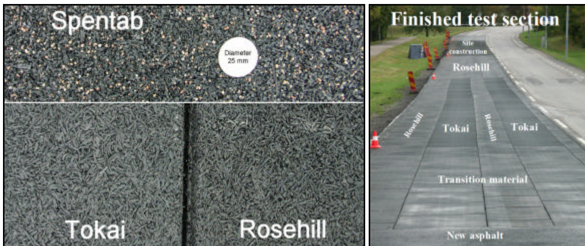
Figure 6.7: Poro-elastic road surfaces trialled in Stockholm, Sweden [111]
