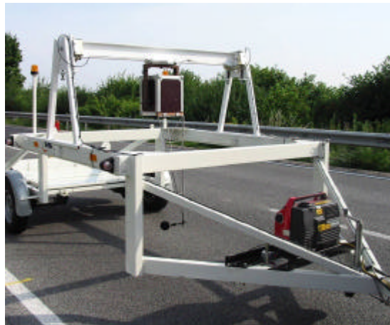
Figure A.15: Mobile MIRIAD system developed by TRL for extended surface method measurements of sound absorption
