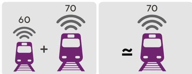
$$60 \text{ dB (A)} + 70 \text{ dB (A)} = 70 \text{ dB (A)}$$
