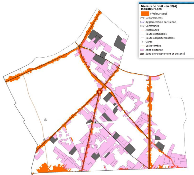
Figure 5 – 2 nd step: Crossing of the "above Threshold values –Roads" map with the "Land use" information
