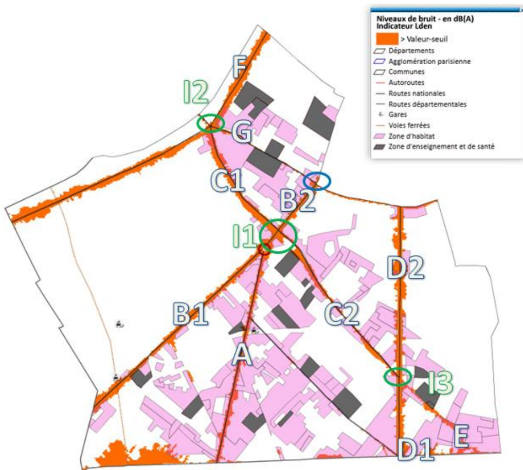
Figure 6 – 3 rd step: Select residential areas or sensitive buildings in areas above threshold values for road noise in Lden
